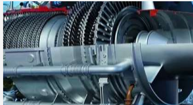
110 MW gas turbine unit as part of a thermal power plant construction project
