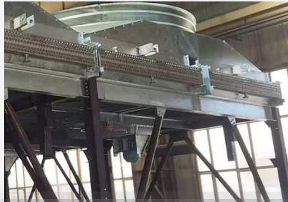
Block-modular air cooling units
