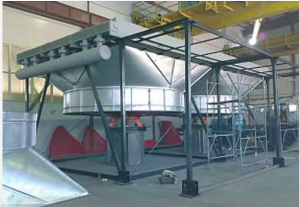
Horizontal air cooling units
